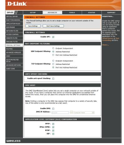
IP Address: Specify the IP address of the computer on the LAN that you want to have unrestricted Internet communication. If this computer obtains it's IP address automatically using DHCP, be sure to make a static reservation on the Basic > DHCP page so that the IP address of the DMZ machine does not change.
