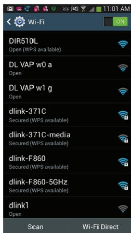
**2** Your device is now connected to the DIR-510L. To connect additional devices, repeat **step 1**.
