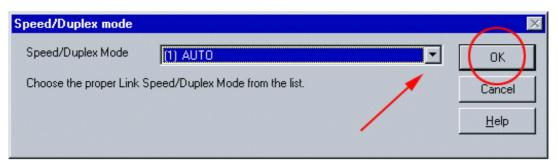
Click "OK" to accept the "Auto" speed mode. To choose a fixed speed mode, make a selection from the "Speed/Duplex Mode" pull-down menu.
