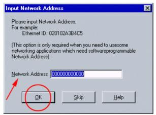
**Click "OK"** if you are not using IPX networking. (Type the IPX network number into the "Network Address" field, if you are using IPX networking.)
