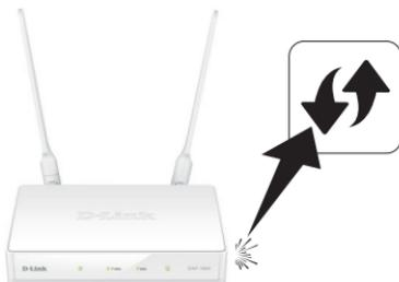
**Note:** For optimal performance using Repeater Mode, place your DAP-1665 in between your router and your dead zone, making sure it's placed in a location where the signal is still strong.
