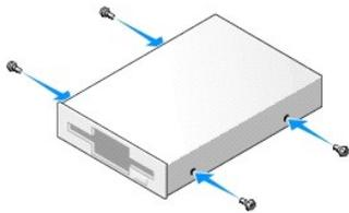
3. Align the shoulder screws on the floppy drive with the shoulder screw slots, and gently slide it into the bay until it clicks into place.
