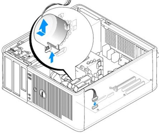
4. Connect the cables to the system board.
