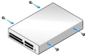
4. Align the shoulder screws with the screw guides, and slide the media card reader into the bay until it clicks into place.
