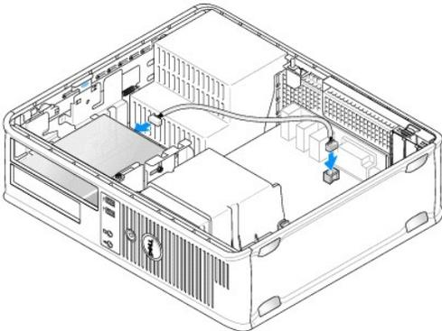
6. Replace the optical drive (see [Optical Drive](#)).
