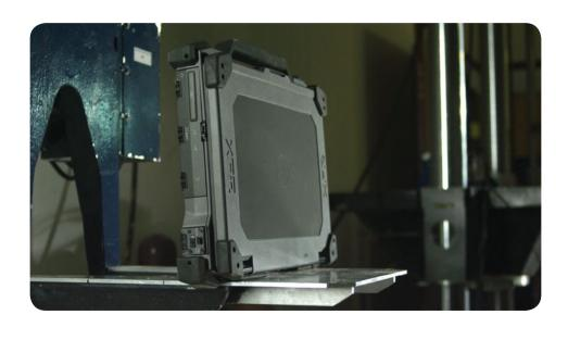
Documented MIL-STD-810G, IEC, UL, emissions, immunity and ESD testing guidelines were followed. All tests were performed with I/O and expansion doors closed. A summary listing of tests appear in the following tables.
