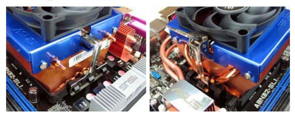
The X-Mars is in no way a large CPU cooler, but the special design of the heatsink can potentially cause installation problems should your mobo's DIMM slots be placed in close proximity to the CPU socket.
