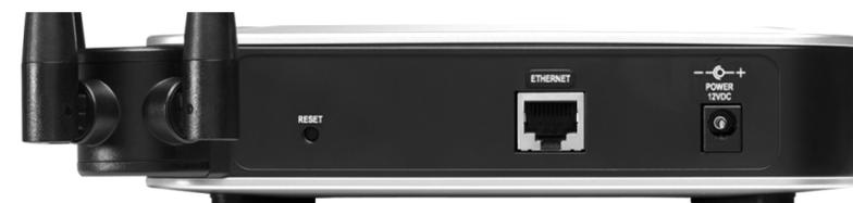
**RESET Button**—There are two ways to reset the access point to the factory default configuration. Either press the Reset button for approximately 10 seconds or restore the defaults using the web-based utility of the access point.
