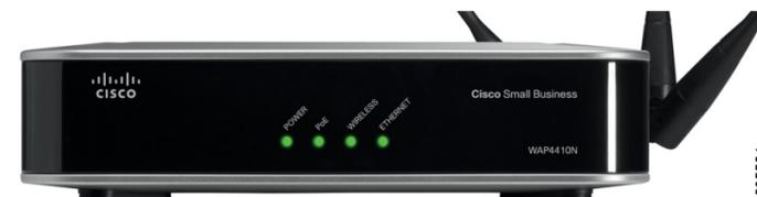
**POWER LED**—(Green) Lights up and remains lit when the access point is powered on.
