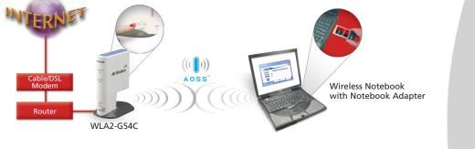
The Wireless Distribution System (WDS) or Bridge/Repeater Mode allows the AirStation to wirelessly communicate with other Buffalo AirStation Access Points (Base Stations) that support WDS. The AirStation 54 Mbps\* Standard Bridge Base Station supports communication with up to six other Buffalo Bridge APs for point-to-point or point-to-multi-point communication and to cover dead zones in WLANs
