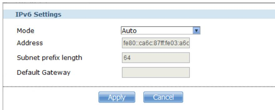
Figure 73. Auto will get IPv6 IP address automatically
