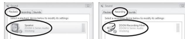
In the "Sound" window, verify that "ZOOM H Series Audio" is listed under the Play and Record devices and that the device is checked. (To switch between Play and Record, click the tabs at the top of the window.)
