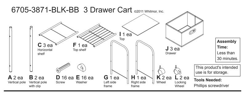
**STEP 1.** Starting with the bottom section, attach vertical poles (A & B) to two horizontal shelves (C) using screws (D) and placing washers (E) between poles and shelf.
