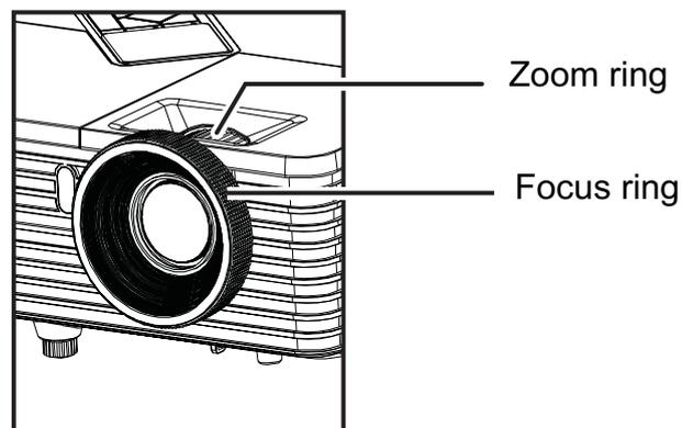
1. Sharpen the image by rotating the focus ring.
