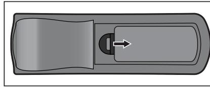
2. Install batteries as indicated by the diagram inside the compartment.
