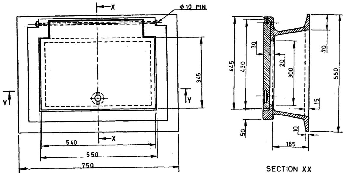
NOTE — The tolerance in dimensions shall be  $\pm 2$  mm for up to and including 15 mm,  $\pm 2$  mm or 16 mm and above and up to and including 50 mm, and  $\pm 5$  mm for 51 mm and above.
