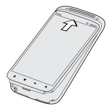
3. Press HTC Sensation 4G down to lock the cover into place. You'll hear a click when the back cover is locked in place.
