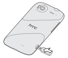
2. Plug in the power adapter to an electrical outlet to start charging the battery.
