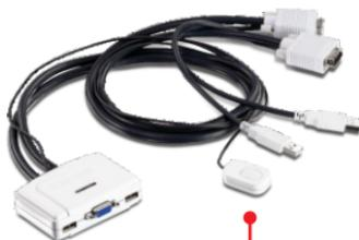
Press the push button switch to switch to the other computer.
