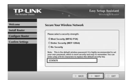
**Note** The Router is pre-encrypted. The default wireless password, the same as the PIN code, is printed on the label at the bottom of the Router.
