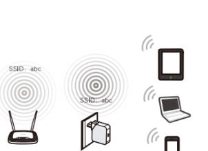
In this mode, this device can be connected to another device via Ethernet cable and act as an adapter to grant your wired devices access to a wireless network, especially for a Smart TV, Media Player, or Game console only with an Ethernet port.
