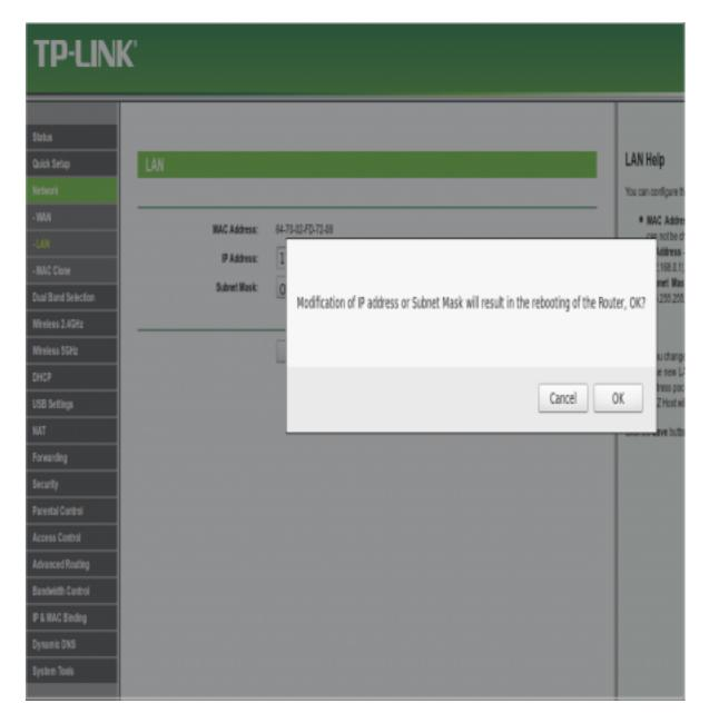
Now the router really, really has to reboot. We're not going to be able to connect to it again until it's functioning as the XSCE's AP. But that's it for the initial configuration.
