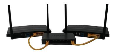
However you can connect the Sharedband routers together with an Ethernet cable (Daisy chained).
