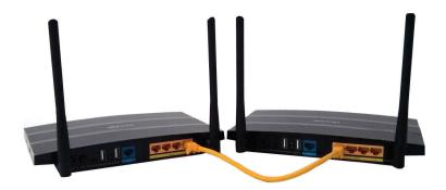
After connecting the Sharedband routers together the next step is to connect the WAN interfaces to your ISP modem/routers. This is done with an Ethernet cable found in the box for each router.
