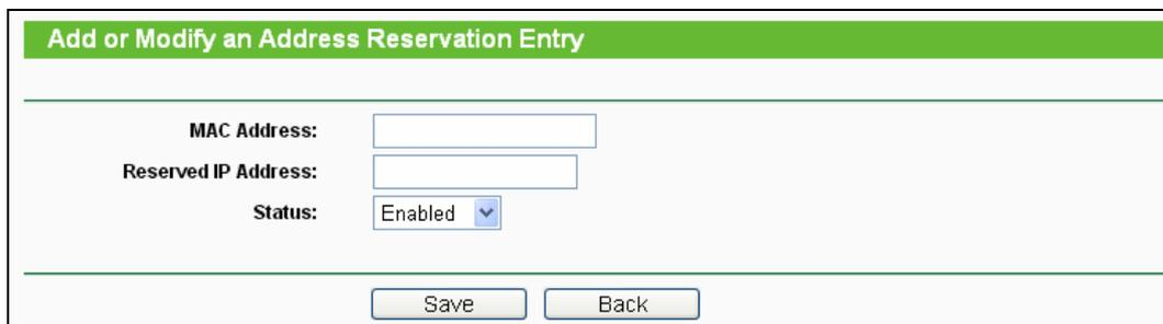
The screenshot shows a web interface for adding or modifying an address reservation entry. It features a green header bar with the text "Add or Modify an Address Reservation Entry". Below the header, there are three input fields: "MAC Address:", "Reserved IP Address:", and "Status:". The "Status" field is a dropdown menu currently set to "Enabled". At the bottom of the form, there are two buttons: "Save" and "Back".
