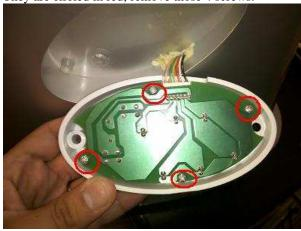
Make sure that the buttons on the board are aligned with the buttons on the white cover.
