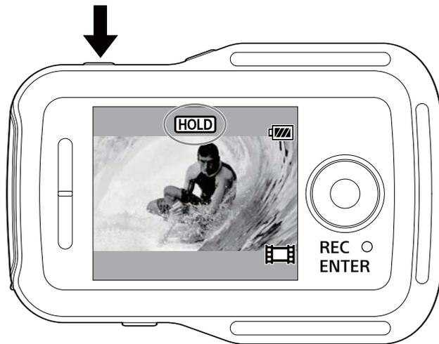
In button hold mode, **HOLD** appears on the LCD screen of this unit. The REC/ENTER button, DISP button, UP button and DOWN button of this unit are disabled.
