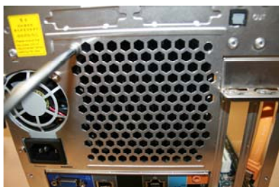
Secure radiator by installing 4 short screws with phillips screwdriver.
