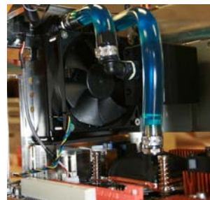
Add thermal paste to CPU Then place cooling unit inside.
