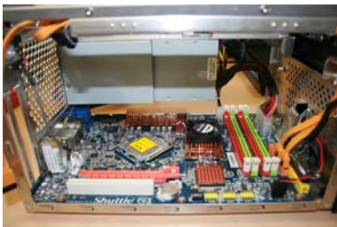
Prep system by removing all current cooling and optical bay bracket.
