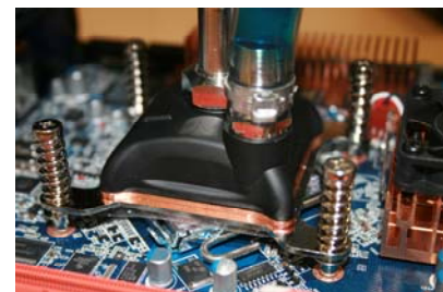
Install and secure CPU water block By using phillips screwdriver .
