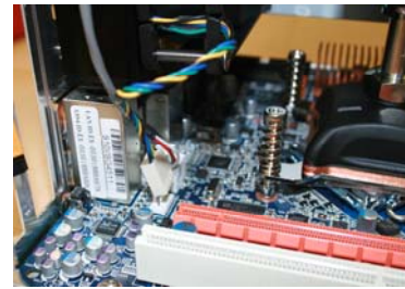
Make sure to install radiator fan power to MB 4-Pin power.
