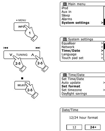
If the 12 hour clock format is chosen, the radio will then use the 12 hour clock for the setting of alarms, and will display a 12 hour clock with an AM or PM indicator when in standby mode.
