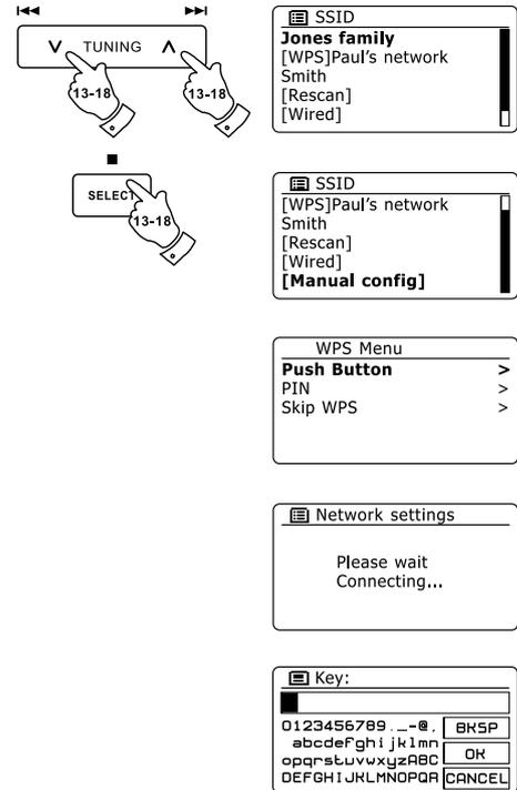
WEP keys are 10 or 26 characters long (using 0 – 9, and A – F). Some wireless Routers can also use pass-phrases for WEP but these are not supported. WPA keys are usually set up using a pass-phrase of between 8 and 63 characters. Your radio accepts pass-phrases for WPA keys.
