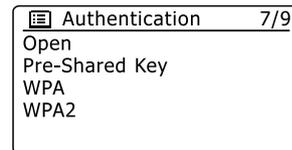
8. If you chose 'Pre-Shared Key' in step 7, you should then choose the WEP option. The key should be entered using only the numbers 0-9 and the letters A-F. The key will be 10 characters long for 64-bit encryption and 26 characters long for 128-bit encryption. The radio will accept lower-case letters a-f as equivalent to upper-case A-F. Spaces or special symbols are not permitted in WEP keys.
