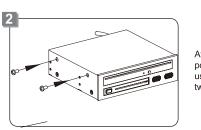
After pushing the slim optical drive into position to align with the front panel, use a magnetic screwdriver to secure two screws to the optical drive.
