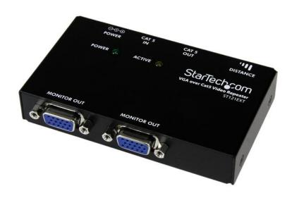
The ST121EXTGB VGA over Cat 5 UTP Video Extender Repeater allows you to further extend your VGA signal over Cat5 or better cabling. This device is specially designed for use with the StarTech.com ST121 VGA Video over Cat 5 extender series, which is comprised of a transmitter unit (ST1214TGB or ST121UTPGB) and an ST121RGB receiver unit.
