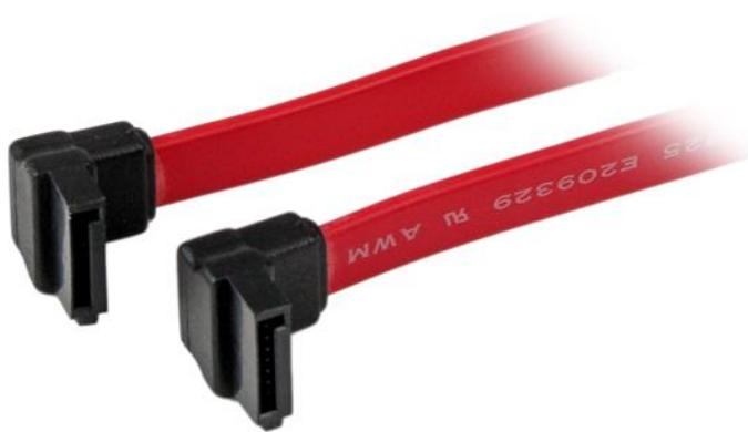
The SATARA18 Right Angle (90-degree) SATA cable (18in) enables you to plug in your SATA hard drive in hard to reach areas or tight spaces, using right-angled SATA connectors to reduce the amount of space required at the connection point and supports full SATA 3.0 bandwidth of up to 6Gbps when used with SATA 3.0 compliant drives.
