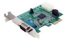
The PEX1S952LP 1 Port Low Profile Native PCI Express RS232 Serial Adapter Card with 16950 UART adds an RS232 (DB9) Serial Port with data rates up to 460 Kbps to a computer through an available low profile PCIe slot, while relying on a native, single-chip design (Oxford OXPCIe952) that harnesses the capability of true PCI Express ensuring maximum performance and reliability and reducing the load applied to the CPU by as much as 48% over conventional (bridge chip) serial cards.
