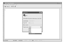
Once the necessary settings have been made, click on OK. The Hyper Terminal window will appear - if all settings are correct, the time clock at the lower left corner of the terminal window will indicate "connected" and the hh:mm:ss timer will begin counting.
