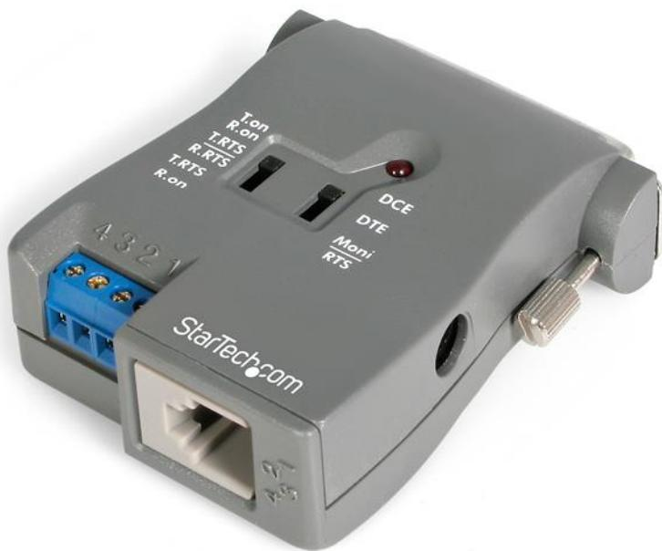
IC485S [IC485SIS] converts RS-232 serial interfaces to RS-485/422 serial interfaces for trouble-free data transmission. This 2-in-1 converter converts RS232C to either the RS-485 or RS-422 interface, and is DCE/DTE mode selectable at the flip of a switch, making it easy to change line signals!
