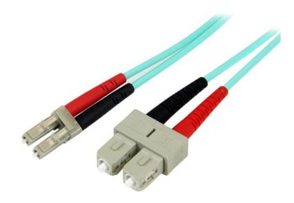
Perfect for fiber cable runs between multiple backbone switches, hubs and routers as well as higher end networking equipment, this high speed 10 Gigabit Multimode Duplex Fiber Cable is terminated with LC and SC connectors, and is composed of 50/125 micron OM3 aqua fiber to deliver reliable data transfers at blinding speeds.
