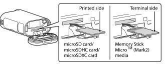
Insert the memory card properly, confirming each side is facing the correct direction.
