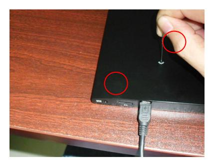
3. Plug in the AC adapter while the reset button is pressed. Your computer will now recognize a different device that is connected to your computer. You may now release the reset
