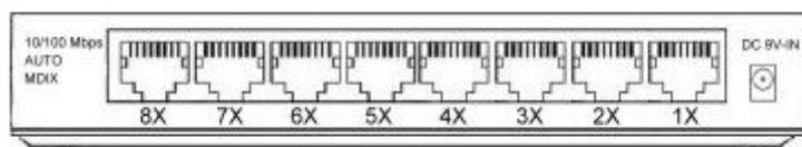
5/8-Port Switch indicates a DC (9V) inlet, which accepts 100-240V 50-60Hz power adapter.
