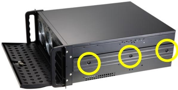
1. In order to install the rail, you must first remove the cover on the side. Three screws locate on each side.
