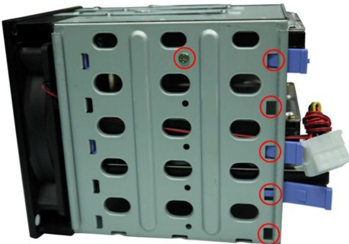
1. Each Hard drive requires using 2x HDD rail on each side.
