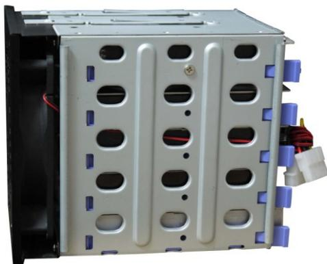
2. The 5x HDDs module should look like this. Each Hard drive is mounted in the module using the HDD rail side by side.
