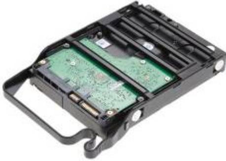
4. The HDD tray can be easily clipped onto 3.5" HDD.
