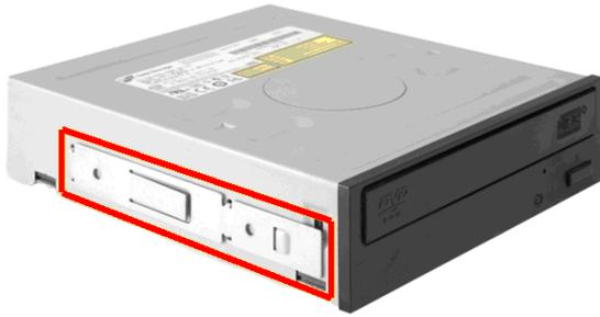
4. Press the ODD rail onto both side of the ODD.
