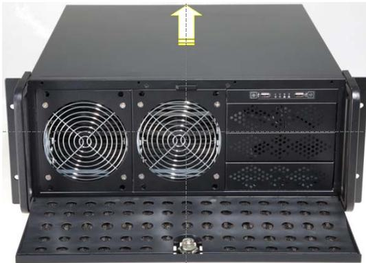
2. Once the screws removed, push the top cover to remove from the chassis.
