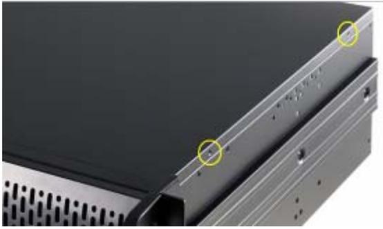
1. Remove the screws from each side of the Chassis. (two on each side)
