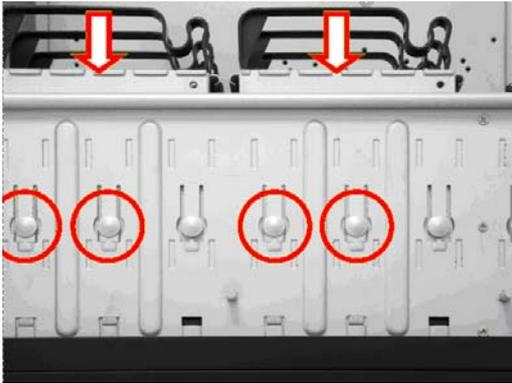
1. First press the two round shape button using your thumbs, then use your index finger to push the middle 3.5" module to remove it.
