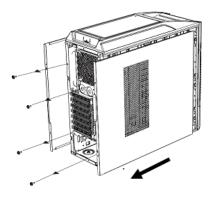
Remove the metal cover plate on the rear of a free PCI slot.
