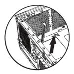
Insert the card into one free PCI slot and screw it firmly on the bracket side.
