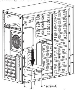
Place 2.5" HDD/SSD onto the bottom of the chassis and secure with screws.
