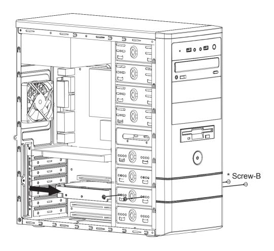
Place the 3.5" HDD into the HDD tray then secure with screws.
