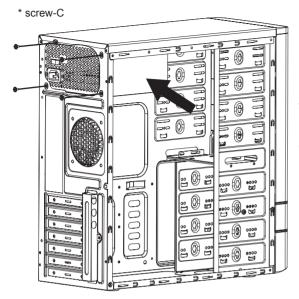
Place the power supply from the left side into the chassis and secure with screws.
