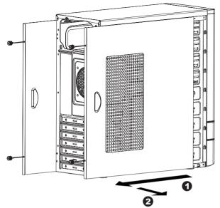
Unscrew to remove left and right panels.
