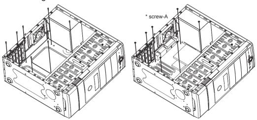
Step 1- Install motherboard stand-offs according to your motherboard's form factor.
