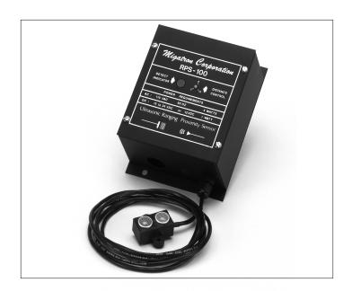
has a broad sensing beam which allows for detection of an object at greater angles of tilt. Sensing ranges available for the RPS-100 include 2" to 14", 5" to 72", and 10" to 240". Mounting flanges, LED indicator, ranging potentiometer, and 6-ft. transducer cable are included. Optional cable lengths are available.
