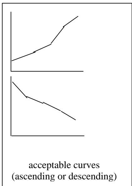
The calibrators' absorbances must be either decreasing or increasing down the strip; i.e., if the first calibrator is the darkest, the second must be the next darkest, etc., and if the first calibrator is the lightest, the second must be the next lightest, etc.
