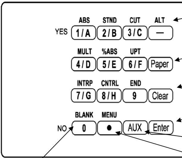
The **ALT** key is used to enter a negative sign and to access a list of alternate functions such as saving and deleting tests, setting the clock, and choosing 8 or 12 well strips.
