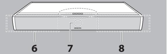
**Regarding the buttons on the main unit:** The buttons on this unit are touch sensitive switches. Therefore, they may respond poorly depending on how they are pressed or not respond when pressed fast and consecutively.
