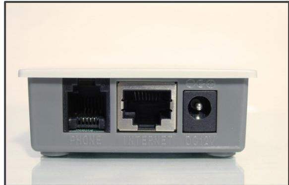
The OBi100 is a dedicated device, built with a high-performance system-on-a-chip platform to ensure high quality voice conversations. The OBi100 has high availability and reliability because it is always-on to make or receive a call. With the OBi100, a computer is not required and a computer does not need to be on to talk to people. To get started, all you need is a phone, power and a connection to the Internet.
