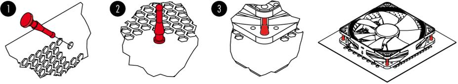
If necessary, you can easily remove the NF-A14 FLX's integrated anti-vibration pads:
