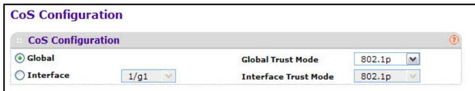
The screenshot shows the 'CoS Configuration' web interface. It features two radio buttons: 'Global' (selected) and 'Interface'. The 'Global' section has a 'Global Trust Mode' dropdown menu set to '802.1p'. The 'Interface' section has an 'Interface Trust Mode' dropdown menu set to '802.1p' and a dropdown menu for the interface name, currently showing '1/g1'. A help icon (?) is visible in the top right corner of the configuration area.
