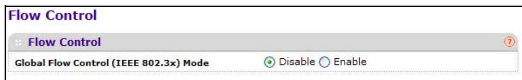
2. Next to Global Flow Control (IEEE 802.3x) Mode, enable or disable IEEE 802.3x flow control on the system. The factory default is Disable.
