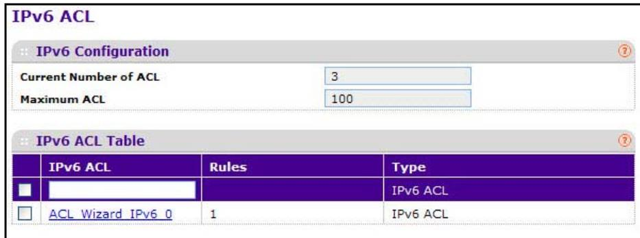
The current number of the IP ACLs configured on the switch is displayed in the Current Number of ACL area. The maximum number of IP ACLs that can be configured on the switch is displayed in the Maximum ACL field, depending on the hardware. The name of IPv6 ACL can be configured in IPv6 ACL field. The number of the rules associated with the IP ACL is displayed in the Rules field. The ACL type is IPv6 ACL and displayed in the Type field.
