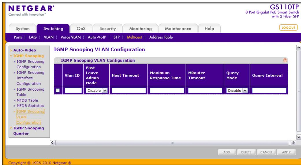
To configure IGMP snooping settings for VLANs:
