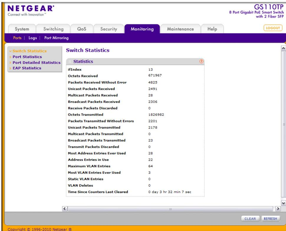
The screenshot shows the Netgear GS110TP web interface. The top navigation bar includes System, Switching, QoS, Security, Monitoring (selected), Maintenance, and Help. The left sidebar shows a tree view with Switch Statistics selected. The main content area displays the Switch Statistics page, which includes a table of statistics and a 'Time Since Counters Last Cleared' field.
