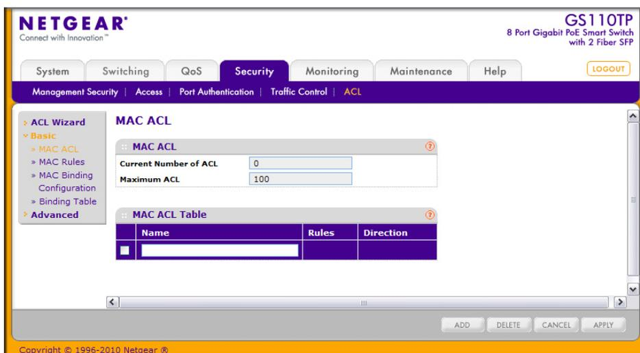
The MAC ACL table displays the number of ACLs currently configured in the switch and the maximum number of ACLs that can be configured. The current size is equal to the number of configured IPv4 ACLs plus the number of configured MAC ACLs.
