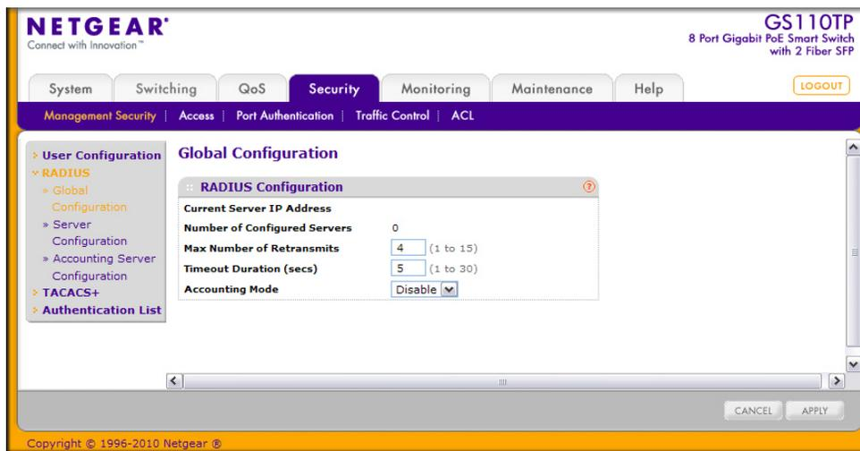
The Current Server IP Address field is blank if no servers are configured (see [RADIUS Server Configuration](#) on page 148). The switch supports up to three configured RADIUS servers. If more than one RADIUS servers are configured, the current server is the server configured as the primary server. If no servers are configured as the primary server, the current server is the most recently added RADIUS server.
