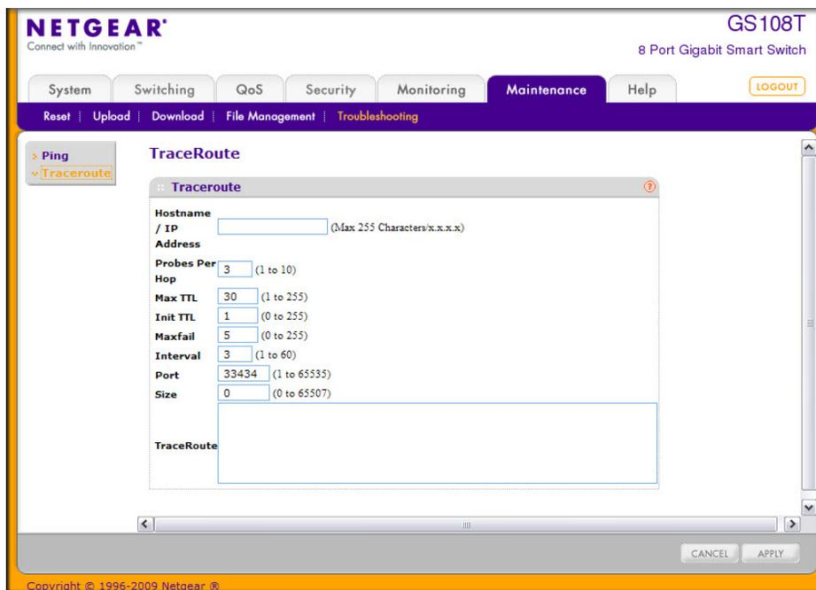
To configure the Traceroute settings and send probe packets to discover the route to a host on the network:
