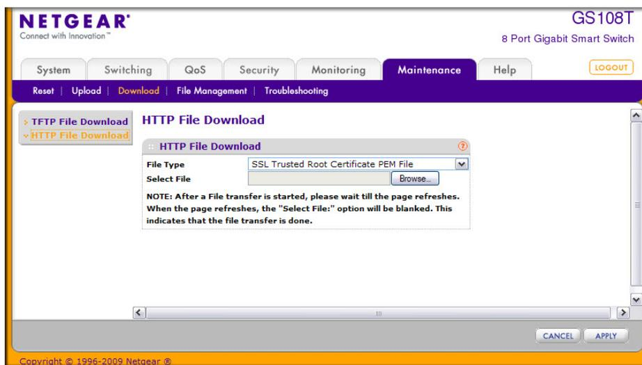
To download a file to the switch from by using HTTP:
