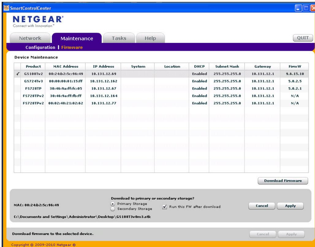
By default, the firmware is downloaded to primary storage and will become the active image after the download completes and the switch reboots. To download firmware to use as a backup image, select the **Secondary Storage** option. To prevent the switch from using the downloaded firmware as the active image, make sure the **Run this FW after download** option is clear.
