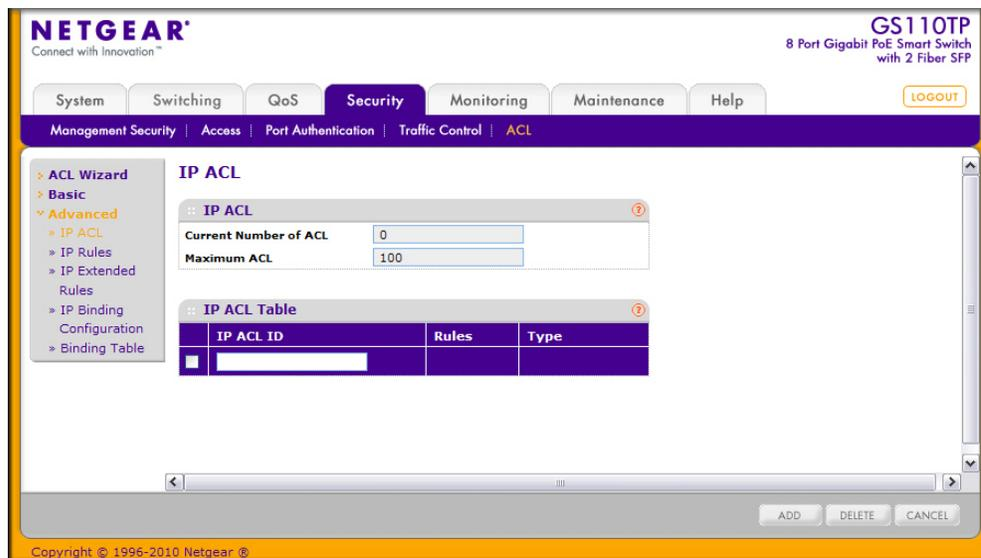
The IP ACL area shows the current size of the ACL table versus the maximum size of the ACL table. The current size is equal to the number of configured IPv4 plus the number of configured MAC ACLs. The maximum size is 100.
