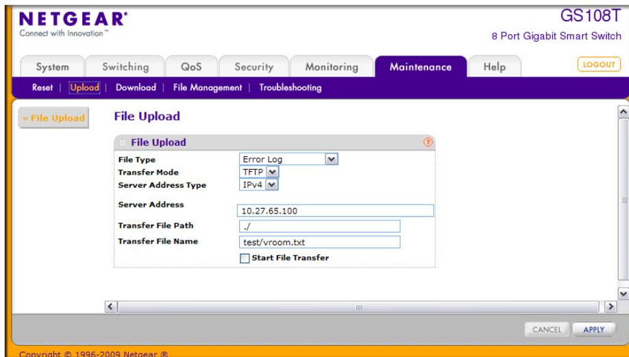
To upload a file from the switch to the TFTP server:
