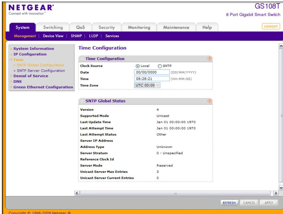
To configure the time by using the CPU clock cycle as the source:
