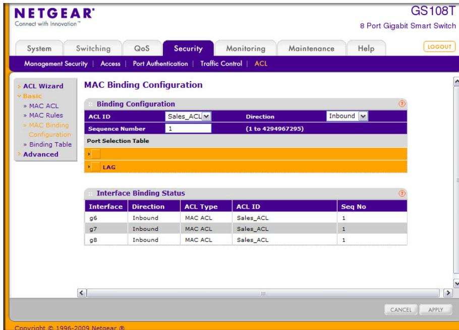
You can assign an optional sequence number to indicate the order of this access list relative to other access lists if any are already assigned to this interface and direction.
