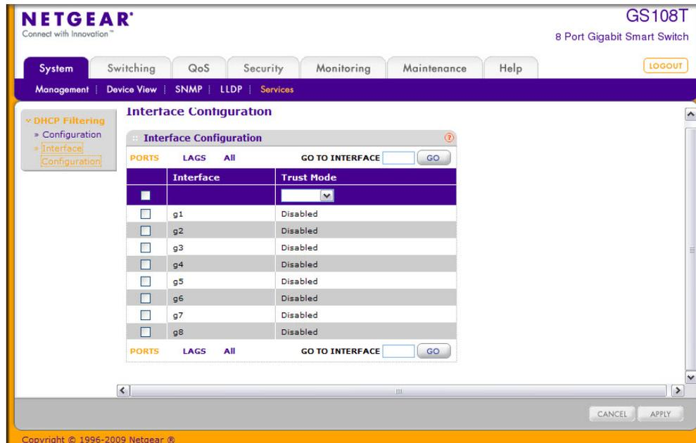
To configure DHCP filtering settings for an interface:
