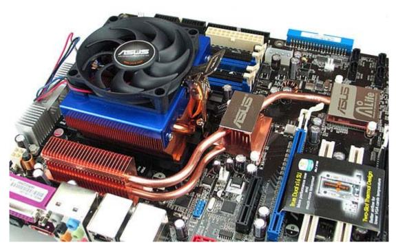
The Heat Pipe design effectively transfers the heat generated by the chipsets to the heatsink near the rear IO ports, where it is carried away by airflow generated by the CPU fan.
