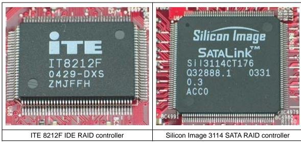
The ITE 8212F controller supports the UltraATA 133 standard and provides two IDE connectors for the support of four IDE devices. Of course, RAID 0/1/0+1 is supported.
