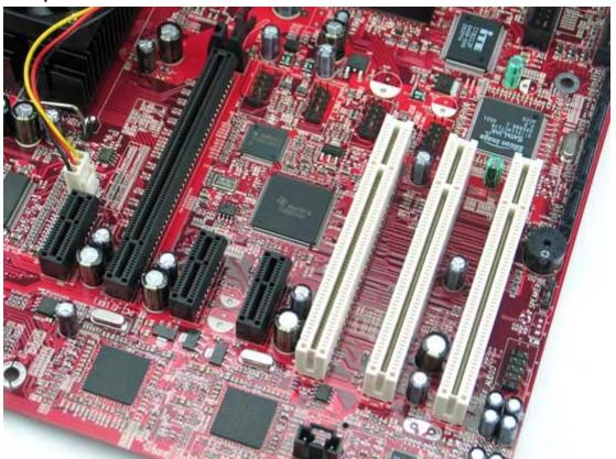
Here we see 1 PCI Express x16 graphics slot being flanked by 3 PCI Express x1 slots. A PCI Express network card means that all 20 of the available PCI Express lanes have been fully utilized. Joining them are 3 PCI slots for standard PCI expansion devices.
