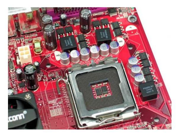
3 phase power solution though it is (hey! Intel's own 925XE motherboards are the same!), each phase is provided with 4 MOSFET so that each MOSFET heats up to a lesser degree. This is a power supply sufficient to deal with the massive demand of Prescott CPUs.
