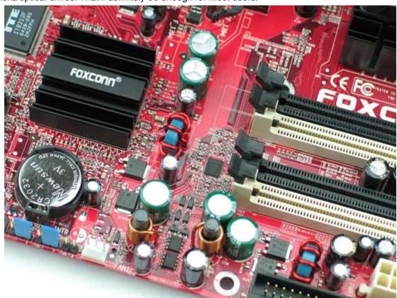
No lack of protection is offered for the PCI Express graphics slot and DIMM slot circuitry as witnessed by the installation of Nippon Chemi-con KZE electrolytic capacitors. This is definitely a power supply level that is sufficient for the PCI Express graphics slot.
