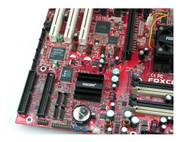
In this picture there are two IDE RAID connectors, 8 SATA RAID connectors, but not the single ATA100 IDE connector that is hidden from view. Together they support a maximum of 14 hard disks/optical drives. That'll definitely be enough for most users.
