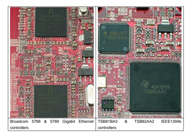
In the left image we have the BCM5788 PCI Gigabit Ethernet controller and the BCM5789 above it, which is a PCI-SIG certified PCI Express Gigabit Ethernet controller that allows heavy bandwidth users to experience the benefits of full-blown Gigabit Ethernet.
