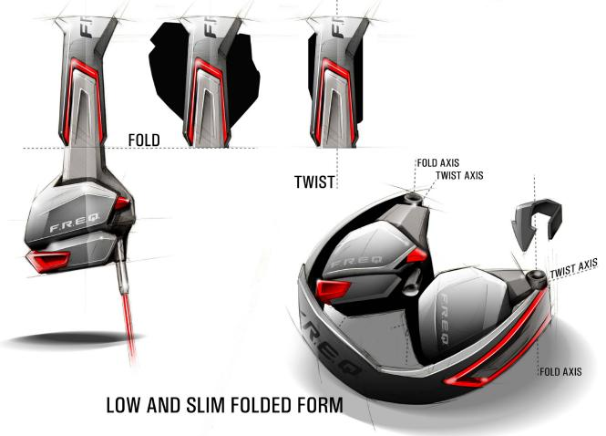
The F.R.E.Q.<sup>M</sup> – like most high-end Mad Catz products – features a very distinctive ergonomic and industrial design. As a travel headset, the F.R.E.Q.<sup>M</sup> will endure some pretty brutal handling at times, so although skeletal in appearance, we precisely engineered each pivot point for strength and reliability. The bi-fold design achieves this objective, yet produces a tiny form factor for easy transportation.
