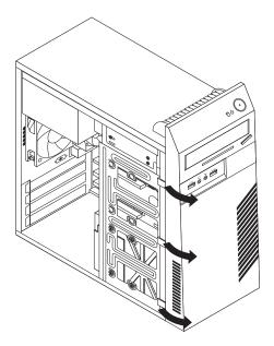
Figure 7. Removing the front bezel
