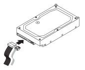
Figure 27. Connecting a SATA hard disk drive
