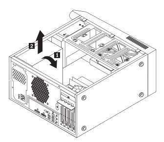
Figure 18. Removing the power supply assembly
