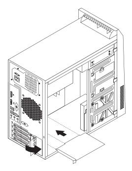
Figure 11. Installing the PCI card
