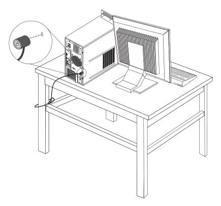
Figure 33. Installing an integrated cable lock
