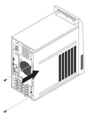
Figure 32. Reinstalling the computer cover
