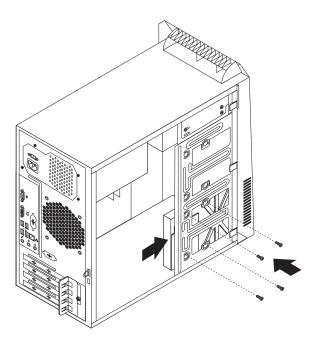
Figure 26. Installing the hard disk drive
