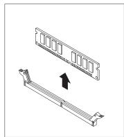
Figure 12. Removing the memory module
