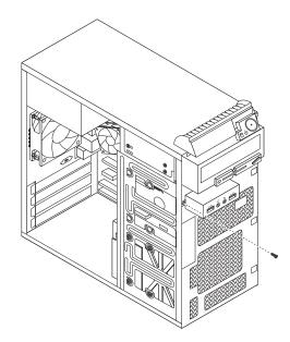
Figure 28. Removing the front audio and USB assembly
