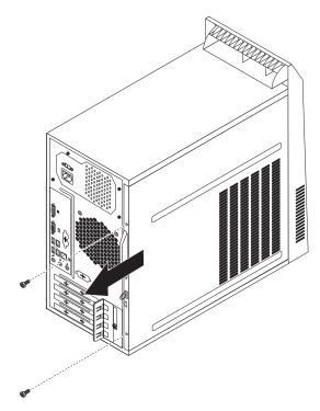
Figure 6. Removing the computer cover
