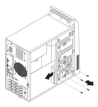
Figure 25. Removing the hard disk drive
