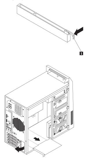
Figure 10. Removing the PCI card
