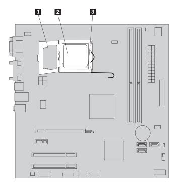
Figure 20. Accessing the microprocessor
