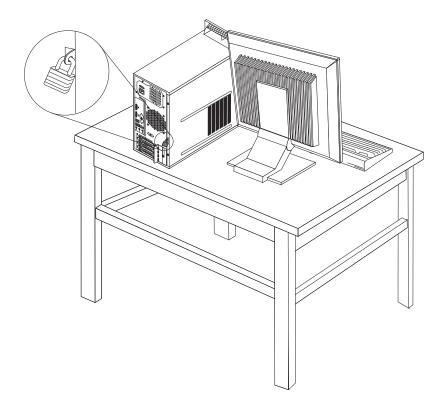
Figure 34. Installing a padlock
