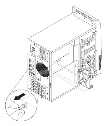
Figure 30. Replacing the rear fan assembly
