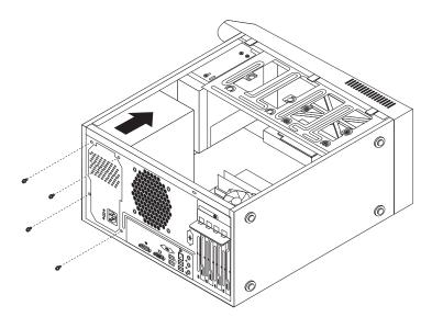
Figure 17. Removing the power supply assembly screws
