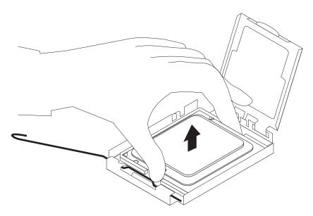
Figure 21. Removing the microprocessor
