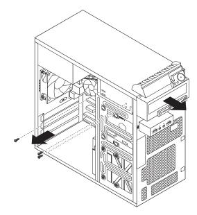
Figure 22. Removing the optical drive
