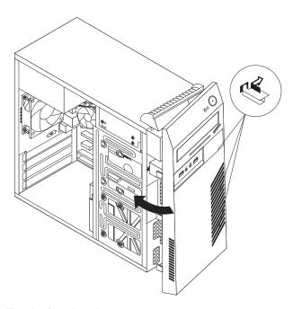
Figure 8. Reinstalling the front bezel
