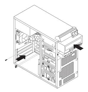
Figure 23. Installing the optical drive
