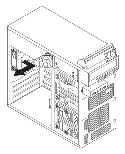
Figure 29. Removing the rear fan assembly
